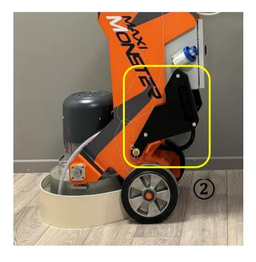
**PHASE 1:** Bring the metal disc close to the female flange connector of the tool holder with the quick-connect pins. Insert the pins of the disc (1) into the slots of the tool holder (2), then turn the disc counterclockwise until it locks.
